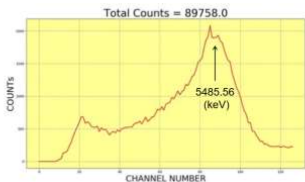
Fig. 7 pixel cluster sizes histogram for ^{241}\text{Am} alpha source. The peak of the distribution corresponds to the maximum energy of incident alpha particles (5485.56 keV).
