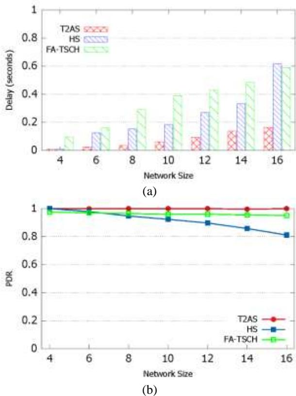
Fig. 9. Simulation results for network with varying size. (a) Average e2e delay w.r.t. network size, (b) Average packet delivery ratio w.r.t. network size.
