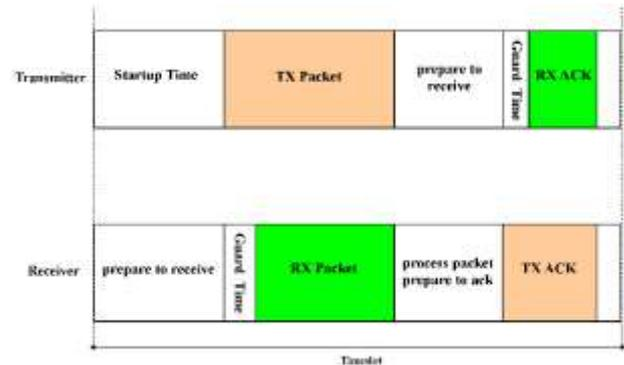
Fig. 2. Structure of a timeslot in TSCH
