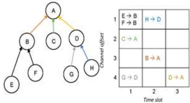
Fig. 1. A sample schedule in a slotframe with 4 channels and 3 timeslots
