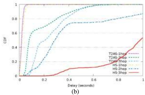
Fig. 7. Simulation results for a 16-node random topology. (a) end-to-end delay, (b) CDF of e2e delay.
