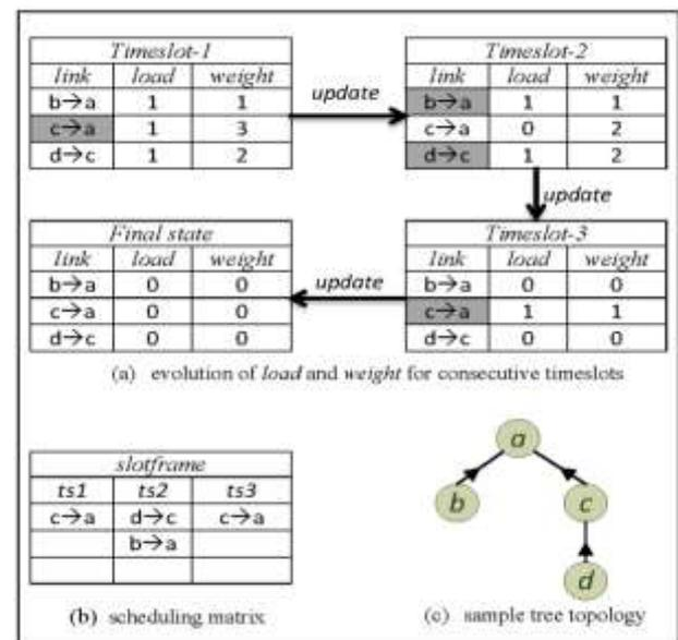
Fig. 4. A sample run for  $T^2AS$  scheduling mechanism Algorithm 2.  $T^2AS$  Scheduling
