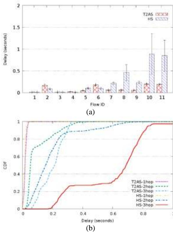
Fig. 6. Simulation results for a 12-node random topology. (a) end-to-end delay, (b) CDF of e2e delay.
